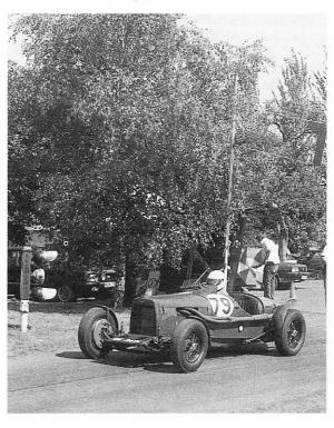
In addition to repainting the car an attractive maroon, Richard Black has continued to develop the special. To date his modifications include replacing the AM gearbox with one from a Riley, lightening the flywheel, and fitting larger SU carburettors with an improved exhaust manifold.
